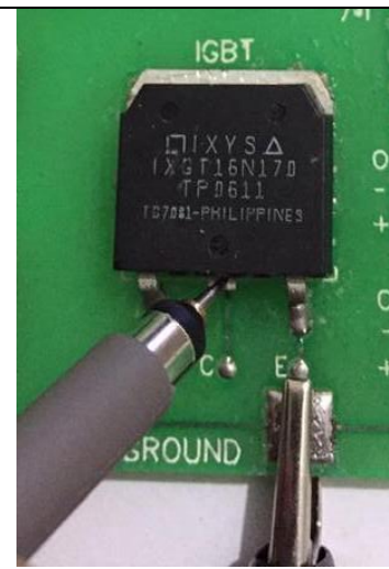
Figure 154: Channel1 Probe Used for Collector - Emitter Measurement
