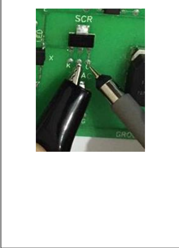
Figure 160: Channel1 Probe Used for Gate - Anode Measurement
