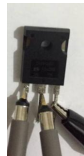
Figure 145: Sample of a Defective N Channel FET
