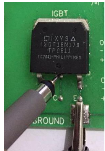
Figure 152: Channel1 Probe Used for Collector - Emitter Measurement
