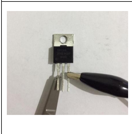
Figure 129: Channel1 Probe Used for Gate - Source Measurement
