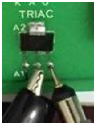
Figure 167: Channel1 Probe Used for Gate - Anode1 Measurement
