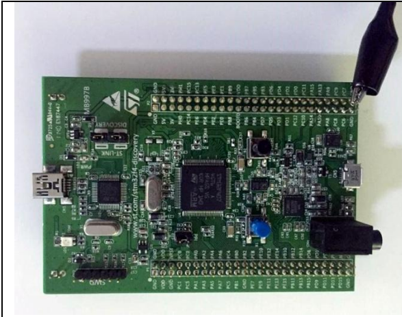
Figure 217: Connecting the Crocodile Probe Electronic Circuit Board Chassis (Step 1)
