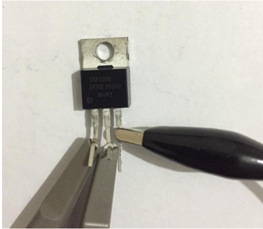
Figure 137: Channel1 (+), Channel2 (+), COM (-) Transistor Test
