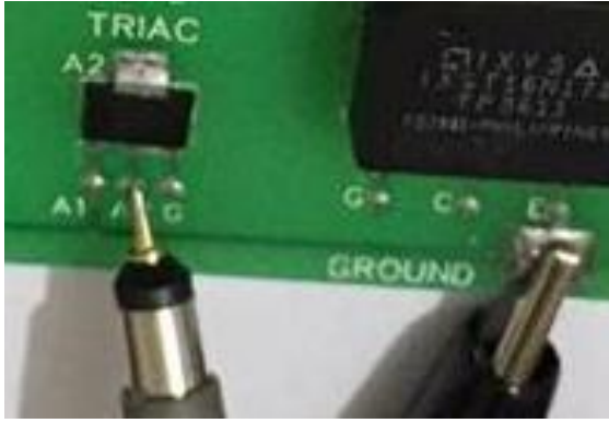
Figure 171: Channel1 Probe Used for Anode2 - Anode1 Measurement
