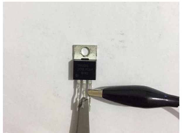
Figure 134: Channel1 Probe Used for Drain - Source Measurement
