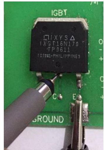
Figure 150: Channel1 Probe Used for Collector - Emitter Measurement
