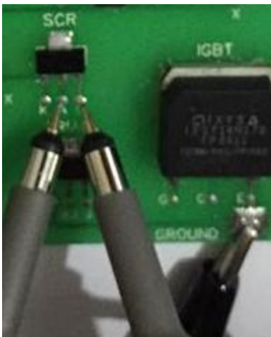
Figure 164: Channel1 (+), Channel2 (+), COM (-) Thyristor Test
