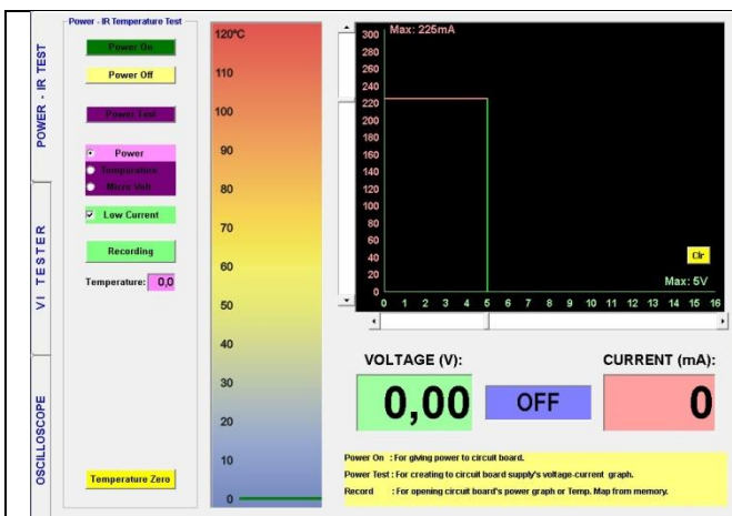
Figure 43: Adjusting the Voltage and Current (Step 1)
