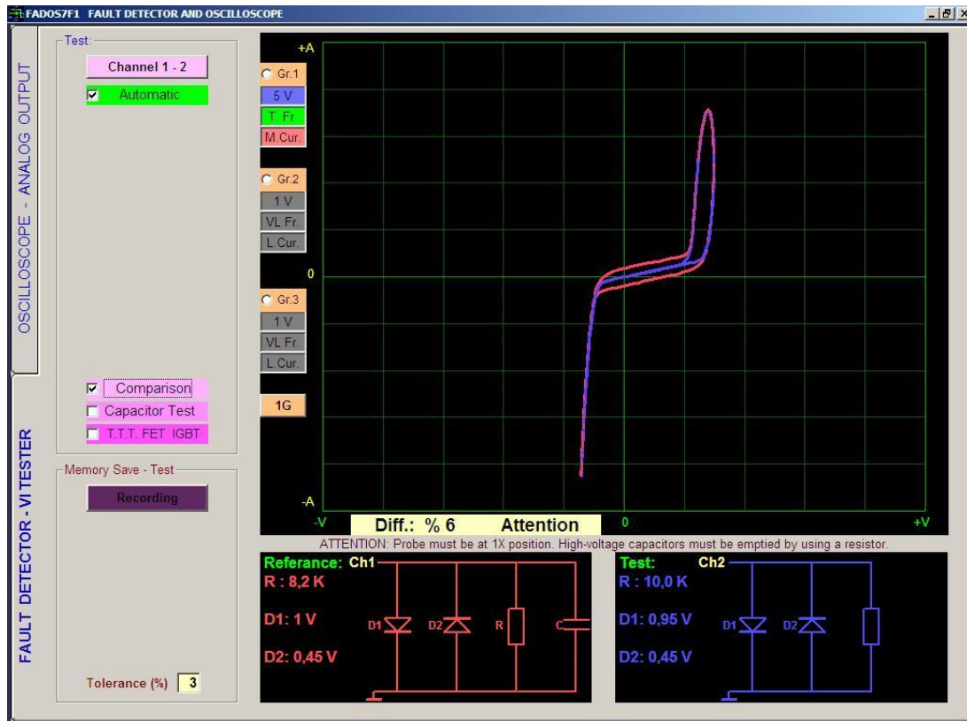
Picture 27: Parallel Capacitor Faults
